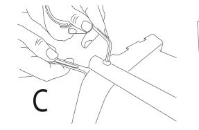
1.4 Push the tubes upwards until they reach the base of the bin and the screws are held in the locating slots at the base of the bin. Tighten the fixing screw and nut using the spanner and allen key provided (diagram C). The sign carrier comprises of a clear rigid wallet, a grey card infill and optional posters.
